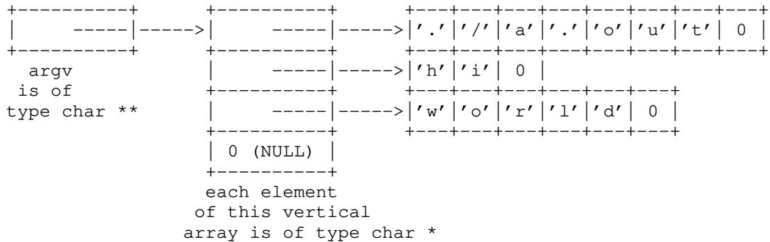
Each element in the vertical array is of type 'char \*' (because they point to the strings on the right.) The argv variable, which points to the first element of the vertical array, is therefore of type 'char \*\*', a pointer to 'char \*'.
