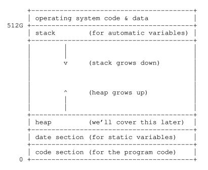
Most computers do not have 512G of physical memory (RAM), let alone enough memory to give 512G to each of the dozens or even hundreds of processes running at any given time. The operating system provides an illusion that each process
