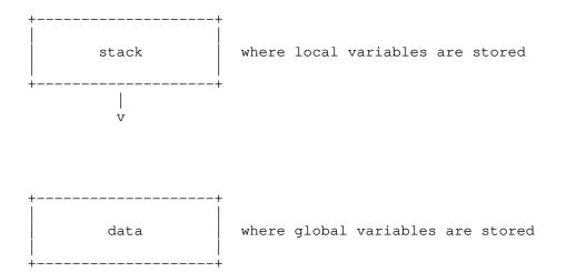
The "stack" stores local variables in each function, and grows downward. Because the number and sizes of global variables stay the same at runtime, the "data" section of memory is fixed at runtime.
